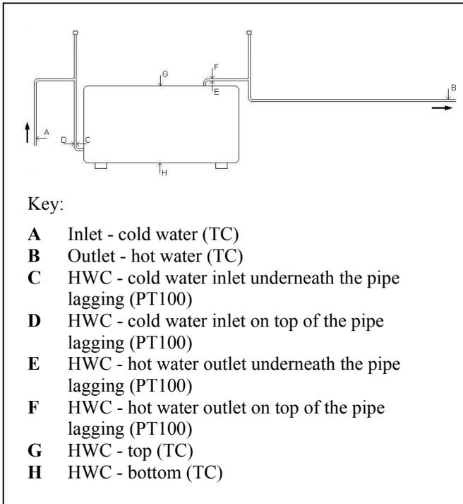
Figure 2 : Positions of the temperature sensors
