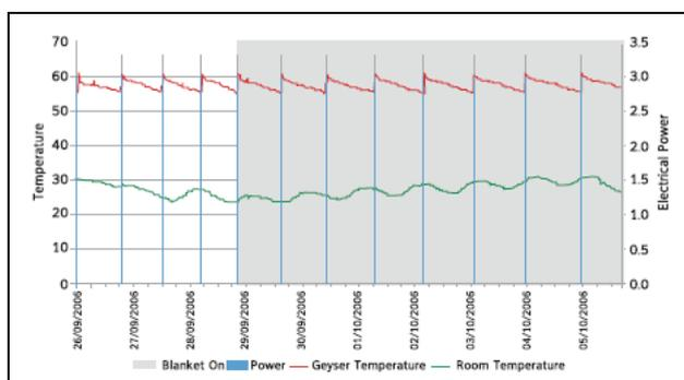
Figure 1: Comparison of geyser and room temperatures with and without a Geyser Blanket [4]
