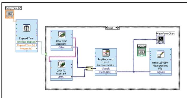
Figure 3 : Block diagram of the ‘Labview’ setup
