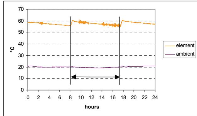
Figure 6 : Temperature gradient over 24 hours of fully covered HWC + Pipes with the element set at 65°C at an average ambient temperature of 20°C.
