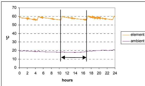
Figure 5 : Temperature gradient over 24 hours of bare HWC and bare Pipes with the element set at 65°C at an average ambient temperature of 19°C.
