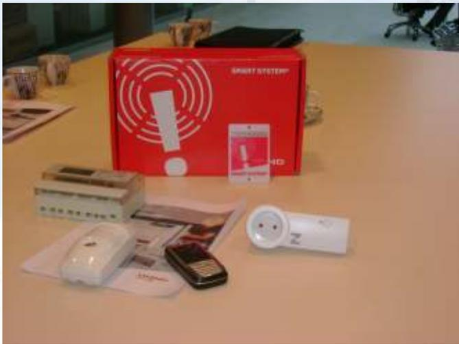
All of the remote devices are connected via wireless communications “ZIGBEE” and are self powered with long life batteries. This means there are no wires and installation is quick and simple.
